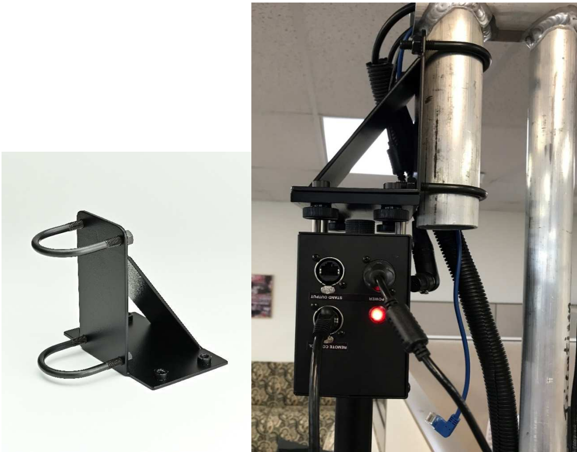
Figure 2 : PTZ Mover with Pipe-grid Ceiling Mount Bracket
