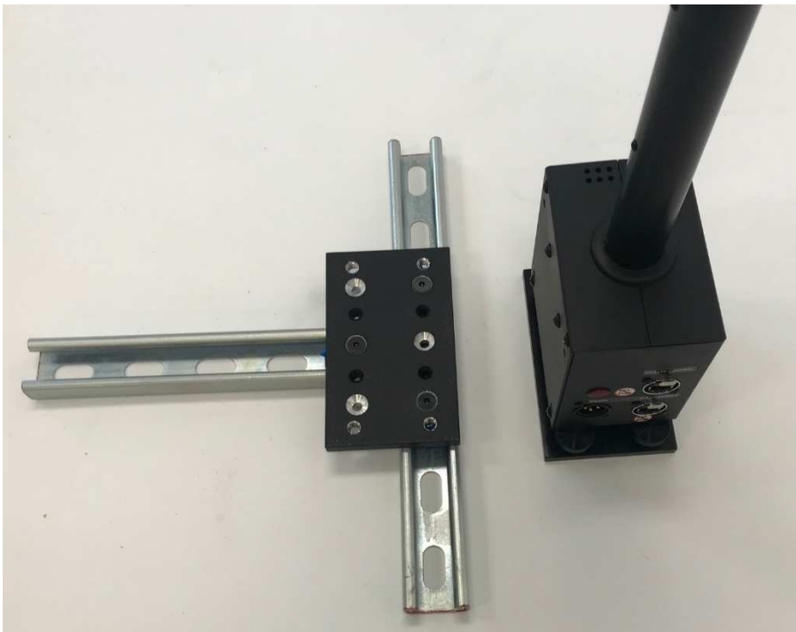
Figure 3 : PTZ Mover with Uni-strut Ceiling mount
